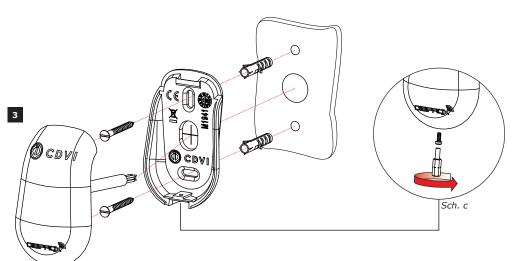
Insert the plastic plugs in the mounting holes, connect the cable (refer to wiring diagram on page 7), then fasten the reader with the TORX® screw using the TORX® bit (Sch. c). Make sure that the varistor is connected across the lock (refer to page 5 "Reminders and recommendations").
